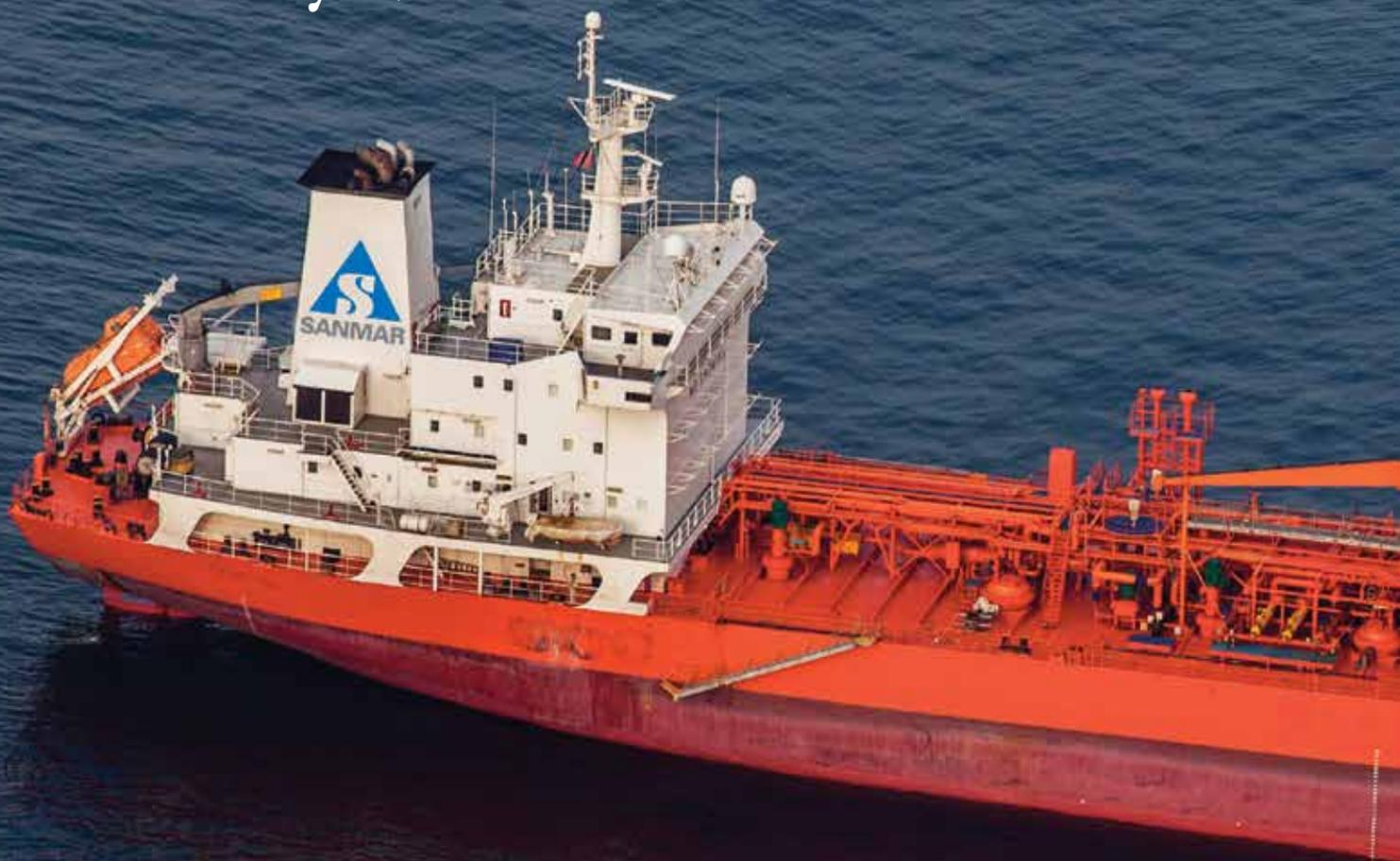
Sanmar Royal, formerly Queen Catalina, the latest addition to the Sanmar fleet, is a Liquefied Petroleum Gas (LPG) carrier, flagged with the Marshall Islands. Being a type C and an ethylene carrier she is one of the most versatile of the gas carriers.
