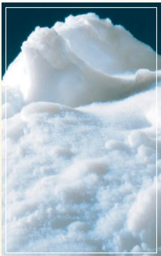
CAB-O-SIL® M-5P fumed silica is hydrophilic due to the presence of surface hydroxyl groups. It has X-ray amorphous structure due to rapid cooling of the silica particles from the molten state to the solid state during manufacturing. It has a refractive index of 1.46 as a result of which it disappears completely in organic solvents having refractive index close to 1.46.
