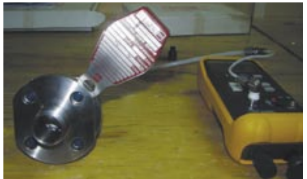
Rupture disks tested by Bloom Energy.
